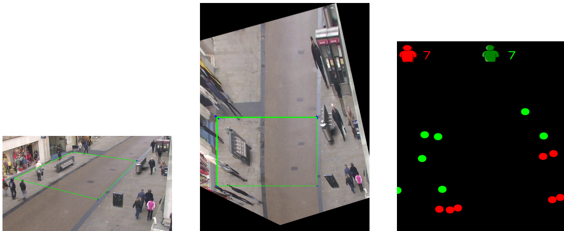
Figure 2.1: 1. Points selection 2. Bird's eye-view transformation 3. Final result
